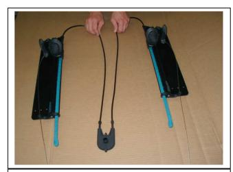
Fig. 7 – Complete Trim Tab and Foot Control assembly laid out.
