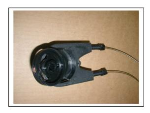
Fig. 6 – Swage slotted into spool.
