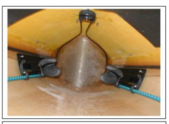
Fig. 1 – View inside kayak with Trim Tab installed.
