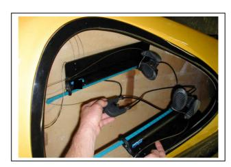
Fig. 8 Insert full assembly into cockpit.
